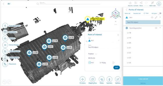
Moreover, this type of POI also offers by default a first person navigation mode in the point cloud at its scanning position.
